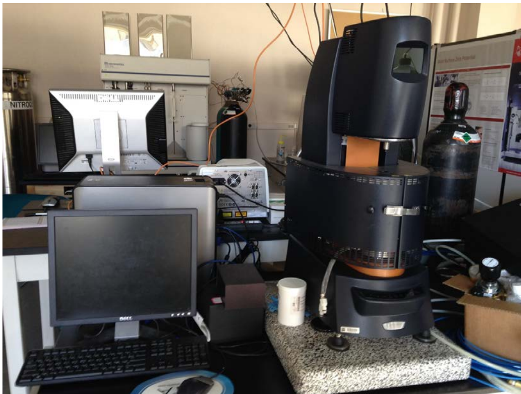
Figure 10. DHR-3 device used for rheometry
