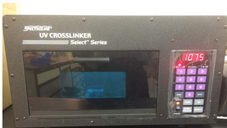
Figure 7. UV cross-linker used to polymerize samples containing photo initiator
