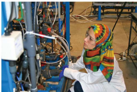
Courtesy photo by Emily C. Kelley Lela Korink, Ph.D. candidate in NMSU's Institute for Energy and the Environment, adjusts the outlet differential pressure on a machine used for brackish water research at Brackish Groundwater National Desalination Research Facility in Alamogordo.
