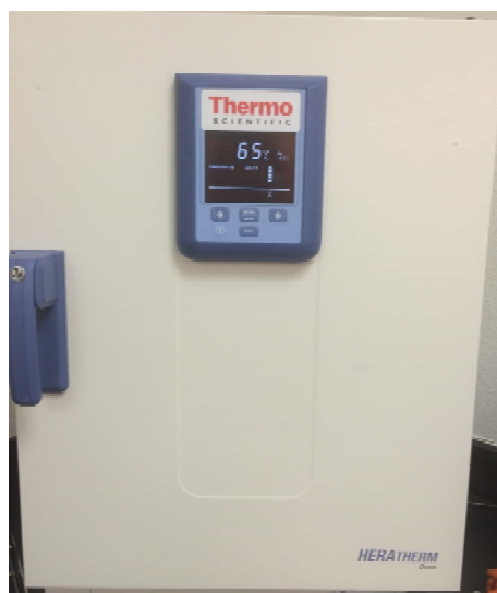
Figure 6. Oven used to polymerize samples containing thermal initiator
