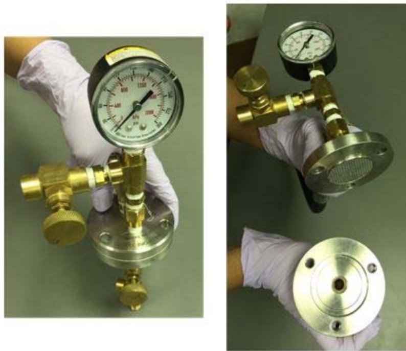
Figure 14. Homemade filtration setup
