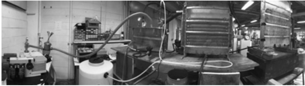
Figure 4.4 Panoramic photograph of fabricated MED unit in the laboratory showing the vacuum pump with cold trap on the left, to the feedwater holding tank, to the MED condenser, second effect, first effect and heat transfer water holding tank on the far right. Photo was taken near the completion of the shakedown trials.
