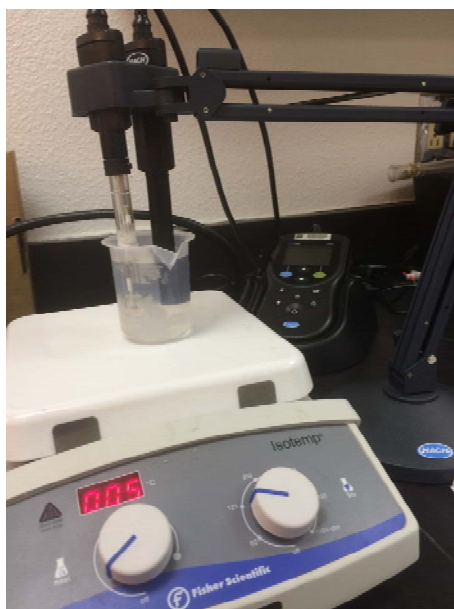
Figure 12. conductometric titration setup
