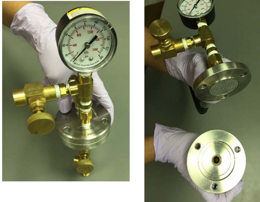
Figure 11. Home-made filtration set-up
