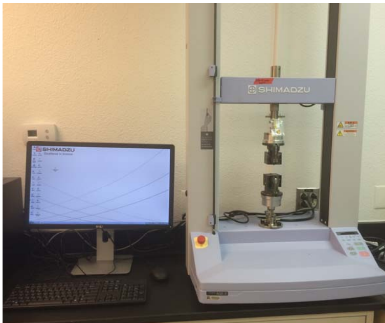
Figure 13. Mechanical tester equipment used to determine the resistance of membranes against pressure
