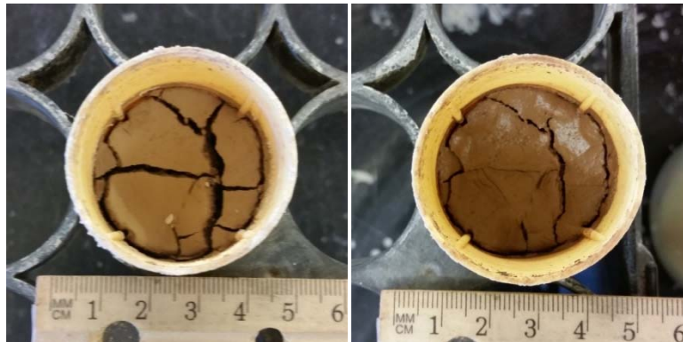
Figure 5 – Cracks formed in clay samples following a drying cycle. All clay samples showed evidence of cracking with drying. On the left, dry clay just prior to concentrate application. On the right, wet clay just after application.
