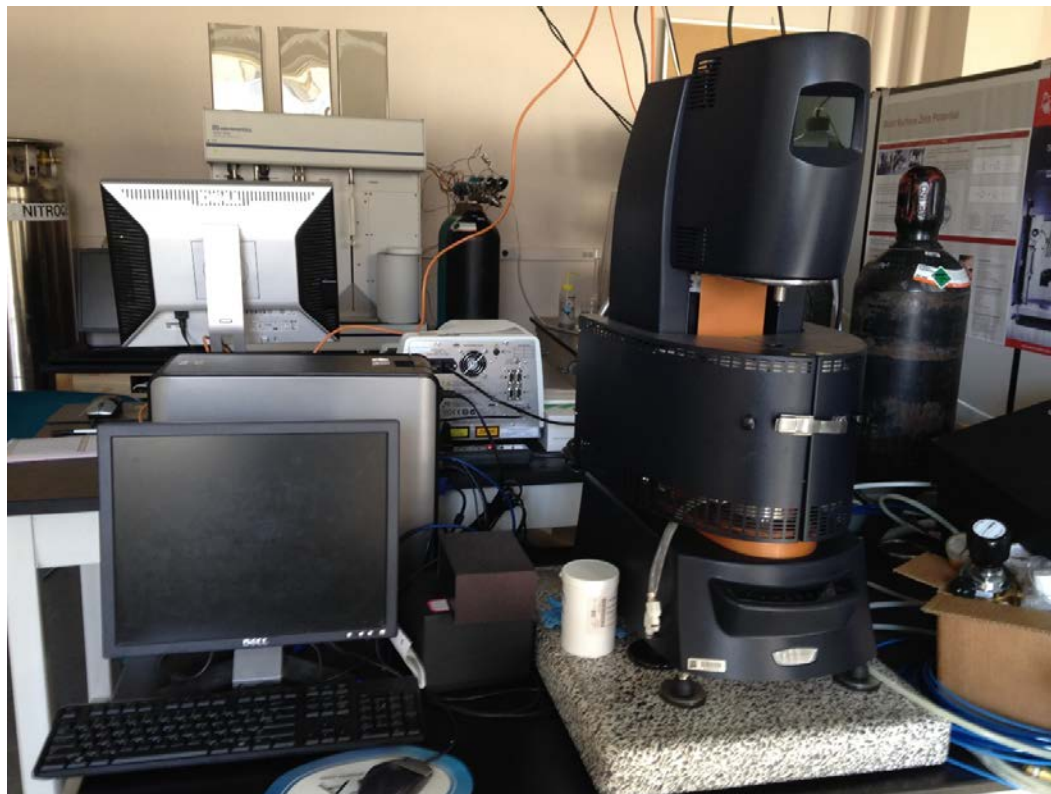
Figure 10. DHR-3 device used for rheometry
