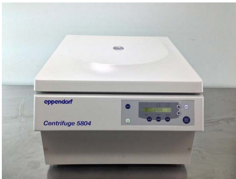
Figure 6. Eppendorf centrifuge model 5804 used for removing talc from permeate
