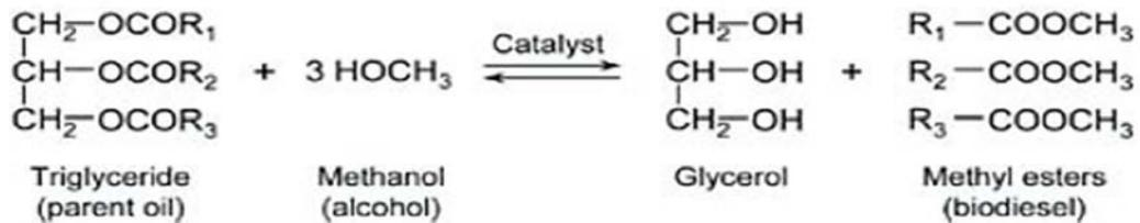
**FIGURE 2.9** Schematic process of biodiesel production
