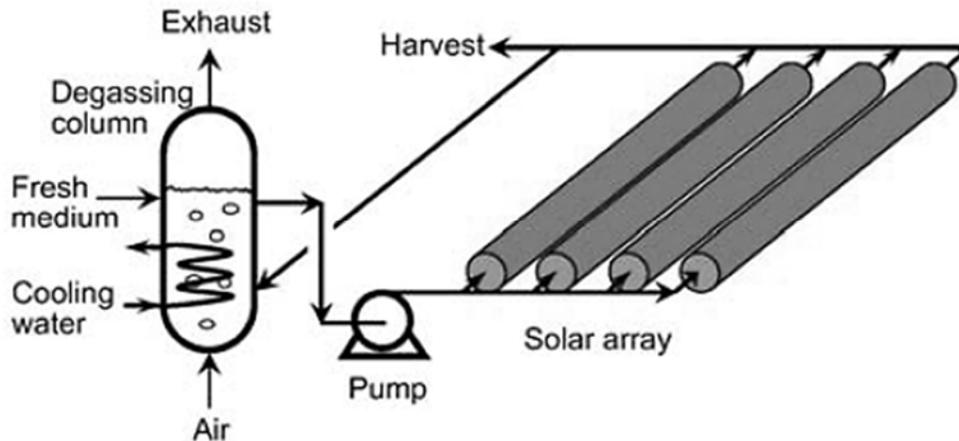
**FIGURE 2.6** A fence-like solar collector
