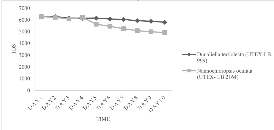
**FIGURE 4.15** Electroconductivity reduction in concentrate medium by two strains of algae
