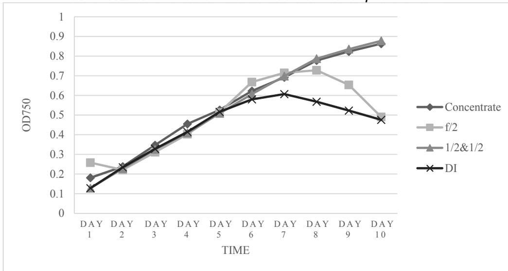
**FIGURE 4.7** Total Nitrogen Removal from concentrate by *Nannochloropsis oculata*
